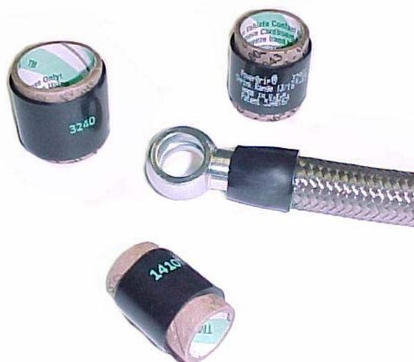
a secure tamper proof connection. We have been using these successfully in a number of nonstandard applications with barbed fittings in different types on hose. They are especially good for keeping stainless overbraided in place - possibly better than a Pro-clamp. Order to hose O.D. - clamps shrink when activated with a heat gun. Other sizes available upon request.
