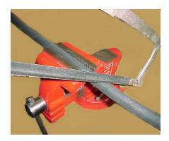
Socketless type hose has no exterior or interior metal braid and cuts easily. Cut hose squarely to length using a fine tooth hacksaw, cable shears, pvc cutter, box knife, or cutoff wheel.
