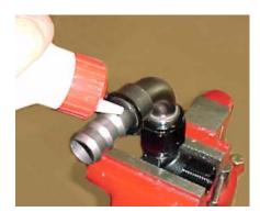
Lubricate both the fitting tail and hose interior where they will come together. Motor oil or liquid soap works well.
