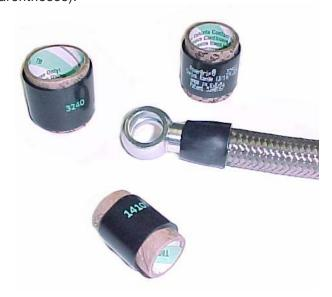
a secure tamper proof connection. We have been using these successfully in a number of nonstandard applications with barbed fittings in different types on hose. They are especially good for keeping stainless overbraid in place - possibly better than a Pro-clamp. Order to hose O.D. - clamps shrink when activated with a heat gun. Other sizes available upon request.
