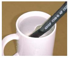
Allowing hose to warm-up will aid assembly; leave in sunlight for a time, or warm some water in the microwave and place the end of hose in to soften.
