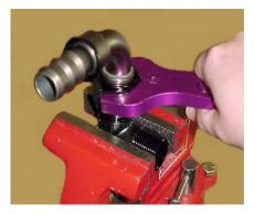
Secure a union in a bench vise and attatch hose end securely. How union is mounted in vise will vary depending on hose angle being fitted.
