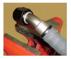
Finished end should resemble this. Hoses with angles at each end can be "clocked" prior to installation. Grip hose and fitting firmly, rotate to proper direction. Hose assembly should be checked for leakage under normal opperation conditions.
