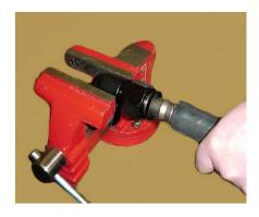
Push and twist the hose over fitting tail until it is tight behind the hose finisher. It helps to do this in one continious motion.
